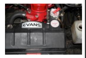
went for it. It expands the usable range from somewhere below zero up to a boiling point around 350 degrees. Also, with no water the rust problem goes away. Well, the change-over day arrived and I flushed the radiator, replaced both hoses and started the preparation process.
