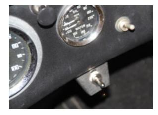
circuit from the light switch and install a separate switch so I can use the LED lights when I need them and turn them off when I don't. Oh well, live and learn. I guess that's the real purpose of owning a Healey anyway.
