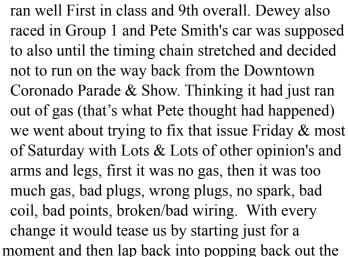
carb, indicating again my original feeling that the timing chain had stretched and the intake valves we still open when the ignition was trying to fire. So, thats racing sometimes, so new adjustable duplex timing chain & gears to the rescue. Thank God Pete had his Formula Ford there to drive as well!!
