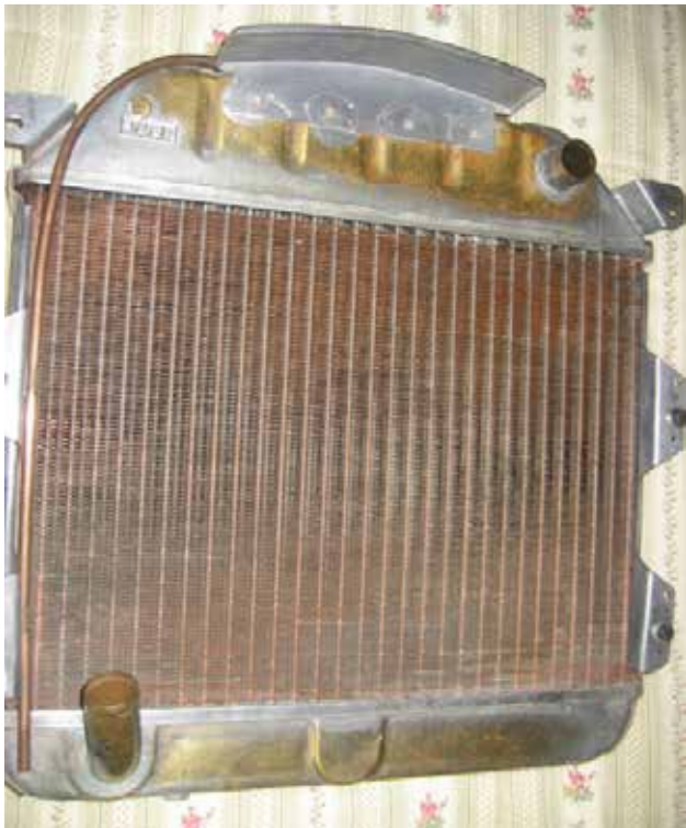
Original radiator core and fins painstakingly straightened w/ fin pliers
