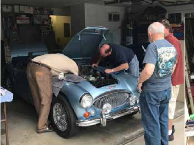
Udo and Don are checking out re-routing the wiring at the old voltage regulator as the alternator has its own.
