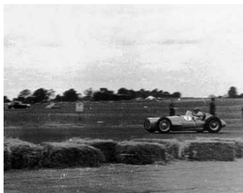
Froilan Gonzales driving a 1500cc BRM V16 at Silverstone in 1953. The BRM had so much power that, when the two stage blowers kicked in, the car would spin it's wheels in top gear. The V16's power surpassed the tire technology of the day.
