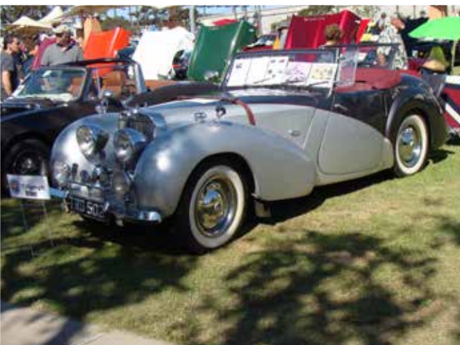
Triumph 2 liter roadster manufactured in 1949. It had an overhead valve engine and a maximum top speed of 65 MPH at 4200 RPM. The engine produced 68BHP. It was the last vehicle made with an occasional Dicky seat. A great looking nice driving around town car.
