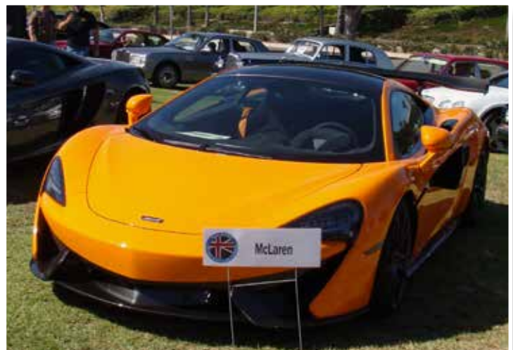
The McLaren 650S has a claimed top speed of 207 MPH and can accelerate from 0 to 60 in 3 seconds. And from 0 to 124 MPH in 8.4 seconds. The engine is a 3.8 twin turbo M838T V8, 7 speed transmission.
