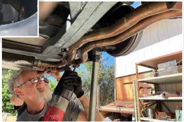
Top- Udo gives Don the bad news. Lou stands by with kleenex. Middle- Gas pump re-mounted to give clearance for right rear shock. Bottom- Udo performs tailpipe surgery with reciprocating saw.
