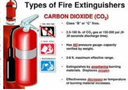
An A class fire is trash, wood, or paper, a B class fire is flamable liquids and grease, and a C class fire is electrical equipment. The extinguishers are also rated by size. There is another class of extinguisher, Class D, but I am not going to discuss this one as it is only used on flammable metal fires, and primarily it is used only in laboratories.
